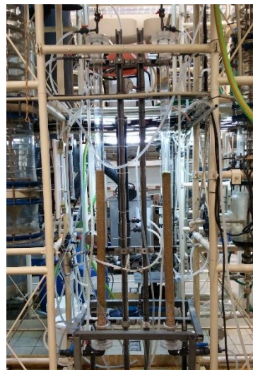
Figure 2 - Fixed bed column with 5.2 cm of diameter
