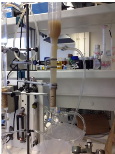
Figure 1 - Fixed bed column with 2,5 cm of diameter
